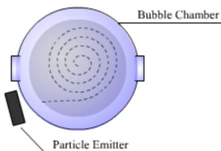
is similar to that of seeding clouds with a chemical to form rain. The idea is that only seeds available in the chamber are those of ions produced by the interaction with radiation. The resulting trail of alcohol droplets can be seen against the black background in the bottom of the chamber.
