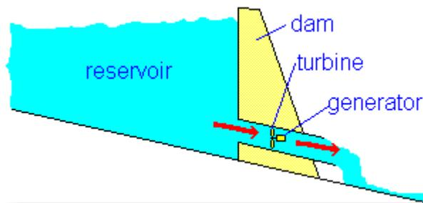
A dam is built to trap water, usually in a valley where there is an existing lake. Water is allowed to flow through tunnels in the dam, to turn turbines and thus drive generators.
