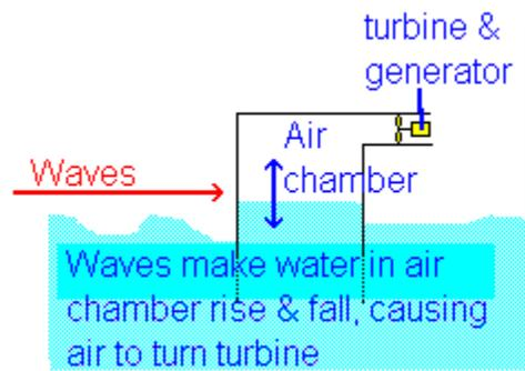
A problem with this design is that the rushing air can be very noisy, unless a silencer is fitted to the turbine. The noise is not a huge problem anyway, as the waves make quite a bit of noise themselves.
